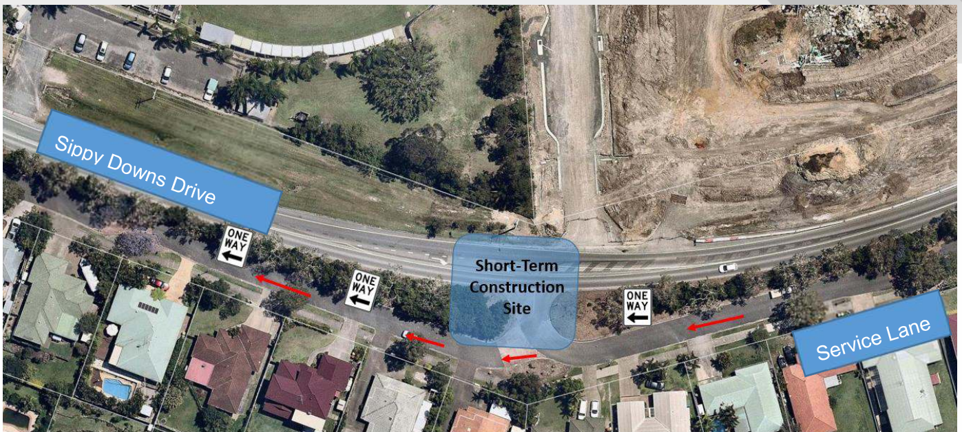
Figure 1 Sippy Downs Drive Service Lane temporary changes to traffic conditions - including temporary construction site, temporary closure of mid-point entry and one way traffic change
